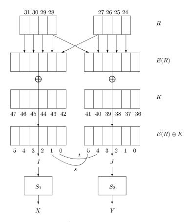
Thus, if s denotes the XOR of  $I_1$  and  $J_5$  (second bit from the right in the first S-box XORed with the first bit from the left in the second S-box), it is by construction of DES a known linear combination of key bits.
